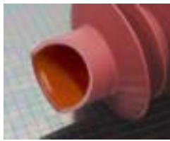
Arrester Housing coated with Mastic
