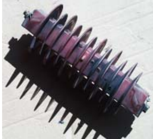
Short-Circuit Test of HDA-NA Surge Arrester arrester prepared with fuse wire according to IEC 99-1 after application of 20 kA short circuit current for 0.2 seconds.
